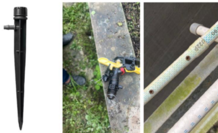
Figure 3 Prototype testing of irrigation components and the development of a low-cost screw adjusted pipe system as a frugal innovation for efficient water management.
